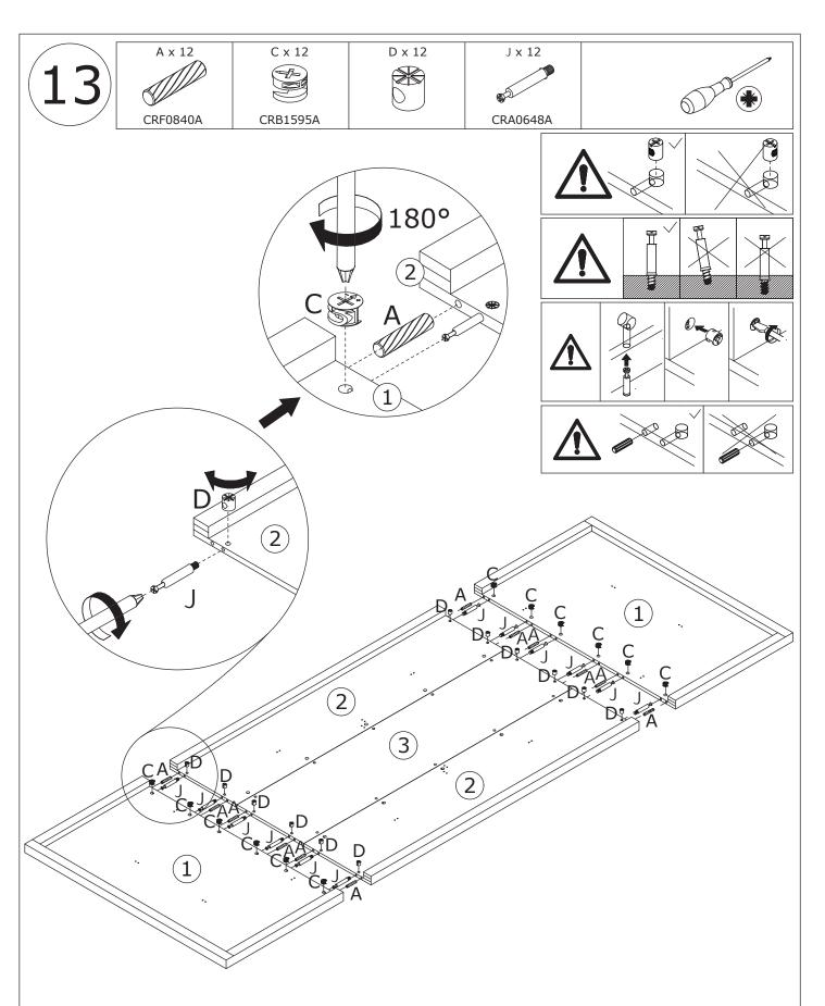
Add nut(D) into panel 2 and 3, and screw eccentric rod(J) into at first. Connect panel 1 to panel 2 and 3 using woooden dowel(A), add cam lock(C) into panel 1 and turn clockwise to tighten as shown.
