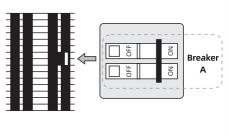
ET008/ET011/ET014: These units can be connected to a single circuit. Use a supply cable protected by a double pole breaker.
