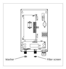
The cold water connection (inlet) is on the right side of the unit, and the hot water connection (outlet) is on the left side of the unit.
