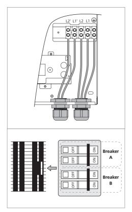
ET018: These units require two independent circuits. Use two supply cables protected by two separate double pole breakers.
