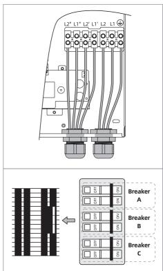
ET024/ET027: These units require three independent circuits. Use two supply cables protected by three separate double pole breakers.
