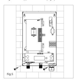
After completing all plumbing and electrical connections, install the front cover and tighten the four upper and lower screws with a screwdriver.
