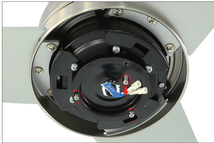
Step 8 Remove 1 screw and loosen 2 screws for the light plate.
