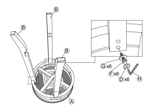
STEP 2 - Tighten the foot ring (C) to leg (B) with JCBC (E) and spring washer (F).
