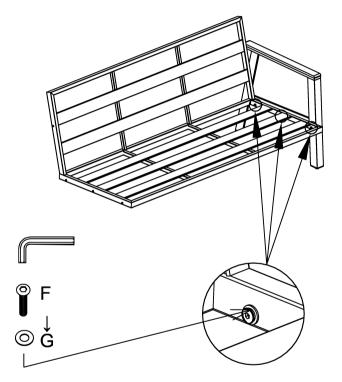
Note:Please do not tighten any bolt until all bolts have been put into right place. If you tighten one bolt, it maybe cause other bolts out of position.
