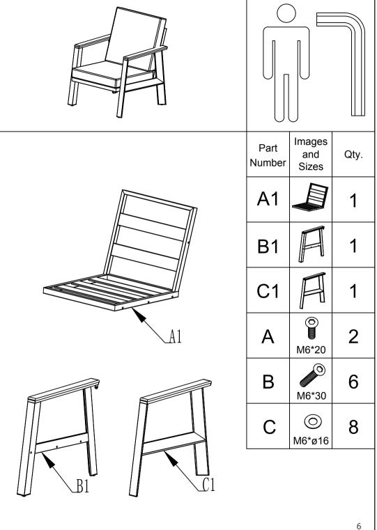
Note:Please do not tighten any bolt until all bolts have been put into right place. If you tighten one bolt, it maybe cause other bolts out of position.
