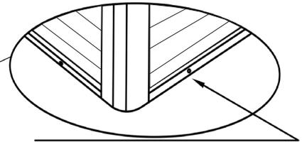
On the outside face, it is suggested to drill holes at the bottom end of the panels to permit drainage when installing on concrete floor /
