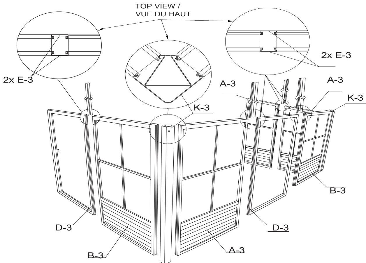
**NOTE:** When placing the door frame opening, make sure the inserts on the frame are on the inside and on the upper half of the frame of the solarium because the door will be set on the inside due to clearance.
