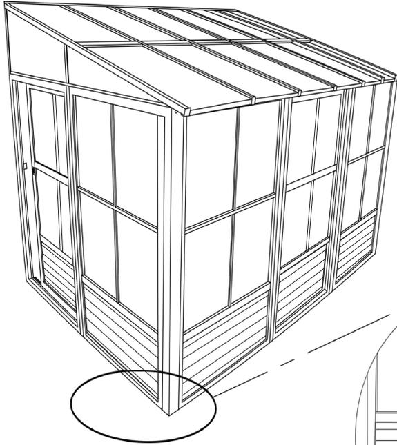
Apply silicone to prevent water from seeping from under the frame /
