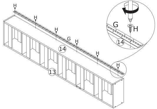
Fix hinge(G) to board 14 with screw(H) as shown.
