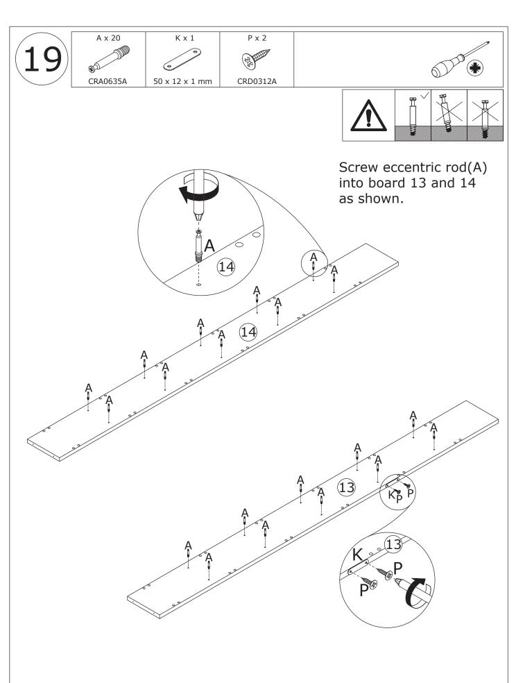
Fix part(K) to board 13 with screw(P) as shown.
