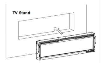
4.4) Fix the firebox with screws(BB).
