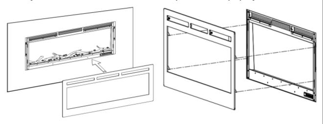
4.9) Fix the glass front by screws (CC) and complete the installation.
