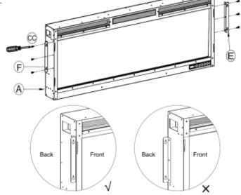
4.3) Insert the firebox into the TV Stand opening, adjust the position of unit and Centered.
