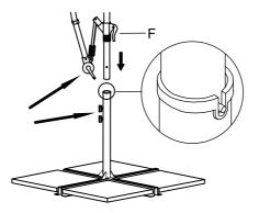
**NOTE:** The central spigot is designed with a reverse angle to ensure the canopy sits level once assembled. It is very important to correctly locate the crank winder directly above the tension screws as shown.
