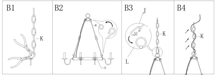
Step B1: By measuring, determine the correct number of links needed for proper hanging height. Using the chain pliers, disconnect and discard the remaining chain.
