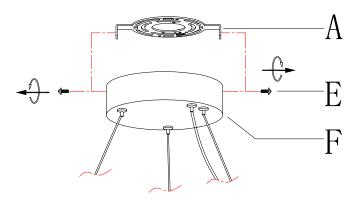
4 » Carefully pass supply wires through mounting plate (A). Secure mounting plate (A) to the outlet box with mounting screws (D).
