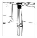
Tighten the two round head screws with a screwdriver.
