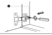
Turn front screw **②** to adjust the gap between the door and cabinet.
