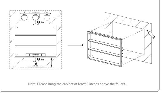
4. Put the medicine cabinet into the cutout opening (1) and mark the spots 1234 for drilling on the wall (2).
