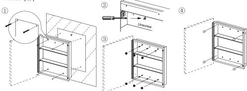
2. Cut the marked perimeter through the drywall (1), remove the cutout (2), and frame the cutout opening as instructed.
