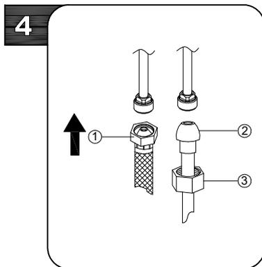
Make connections to water lines. Use 1/2" I.P.S. faucet connections (1) or use coupling nuts (3) with 3/8" O.D. ball-nose riser(2). Use wrenches to tighten connections. Do not overtighten.
