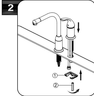
Place handle assembly through side hole in sink. Secure handle assembly with washer (1) and nut (2). Make sure that the slot on nut is facing up. Make sure handle is facing forward and it swings equally in both directions.
