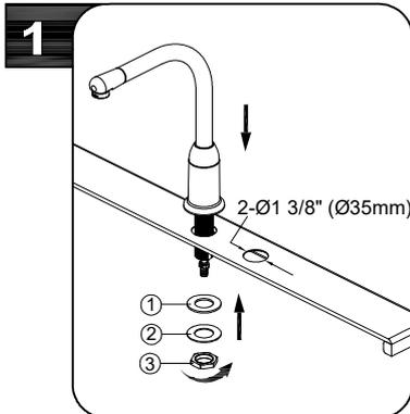
Shut off water supplies. Place spout through mounting hole in sink. Secure spout with rubber washer (1), metal washer (2) and nut (3).
