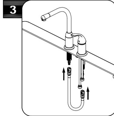
Attach the hose to the connection beneath the faucet by aligning the tabs on quick connectors. Push quick connectors housing firmly upward and snap onto receiving tube tabs. Pull down moderately to ensure connection has been made. If it is necessary to remove the quick connectors, squeeze tabs on hose between index finger and thumb, then pull down to disconnect.
