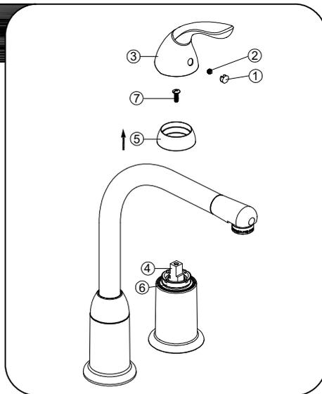
Shut off water supply. Remove set screw plug (1). With valves in "closed" position, unscrew set screw (2) and remove handle (3) from valve stem (4). Loosen the screw (7) from valve stem (4). Loosen the cap (5) from the cartridge nut (6).
