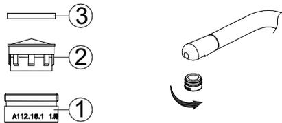
This faucet ships with a 1.5GPM aerator installed. An optional 2.2GPM aerator is also included in the box.
