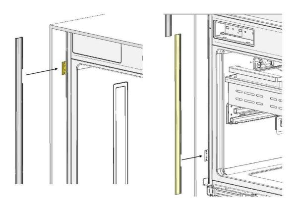
• Attach the upper closing part (4) onto the upper connection bracket.
