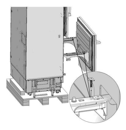
Pull the door frontward to free it from the tabs at the back and remove it.
