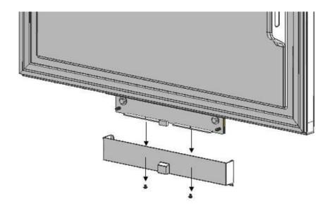
Remove FF Lower and Upper Bracket screws.
