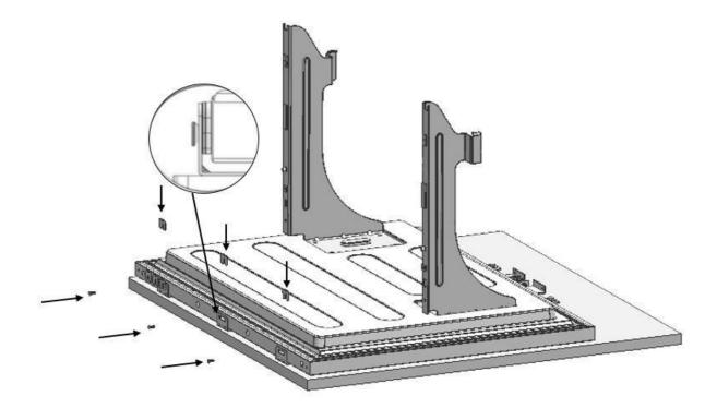
A total of 3 mm washers must be placed on the FRZ Door on the condition that all furniture dimensions are suitable.
