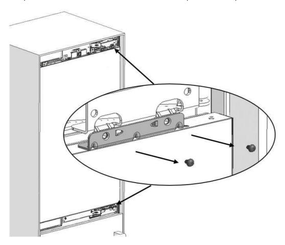
Take out the FF Door and lay it down on a table remove the fixing parts and screw them to the opposite side of the door.
