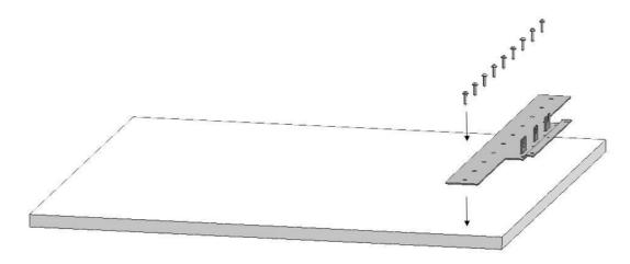
• Attach 3 sheet metal brackets (Item No14) using 6 screws (Item No15) for each.
