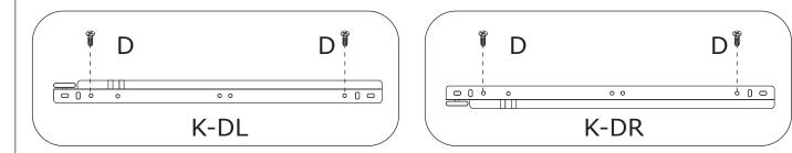
Fix runner(K-DL) and (K-DR) to board 19 and 23 respectively with screw(D) as shown.
