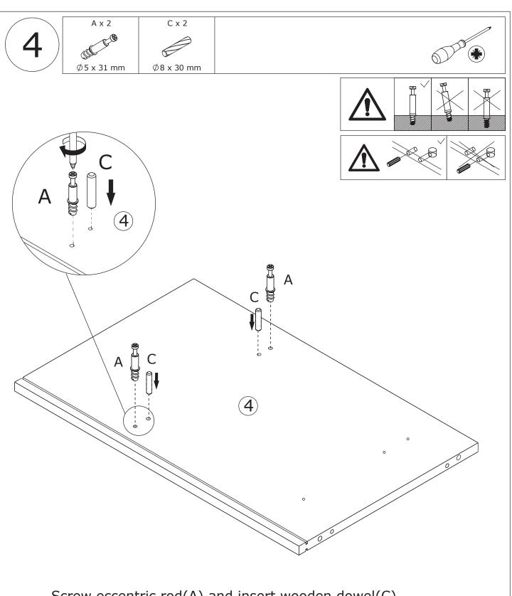
Screw eccentric rod(A) and insert wooden dowel(C) into board 4 as shown.
