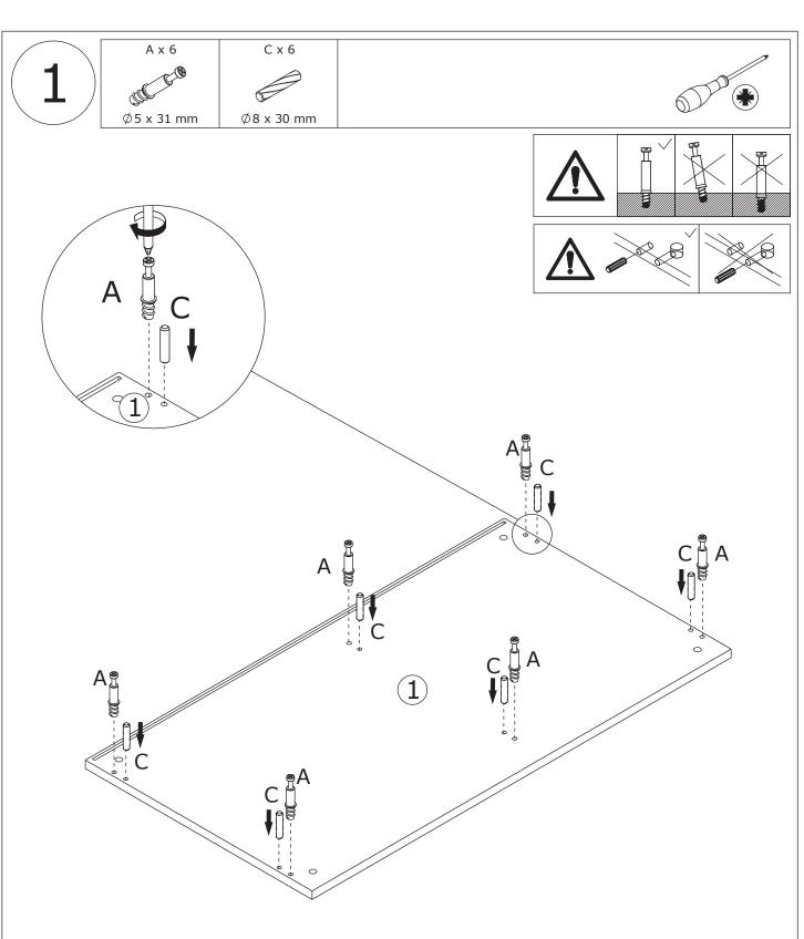
Screw eccentric rod(A) and insert wooden dowel(C) into board 1 as shown.
