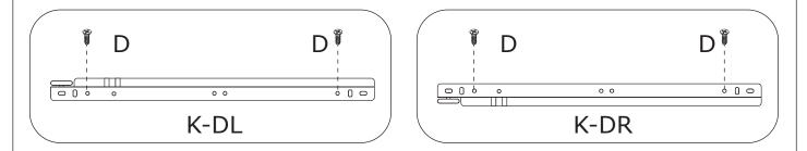
Fix runner(K-DL) and (K-DR) to board 25 and 27 respectively with screw(D) as shown.
