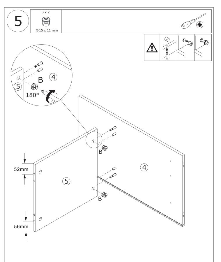
Attatch board 5 to board 4, add cam lock(B) into board 5 and turn clockwise to tighten as shown.
