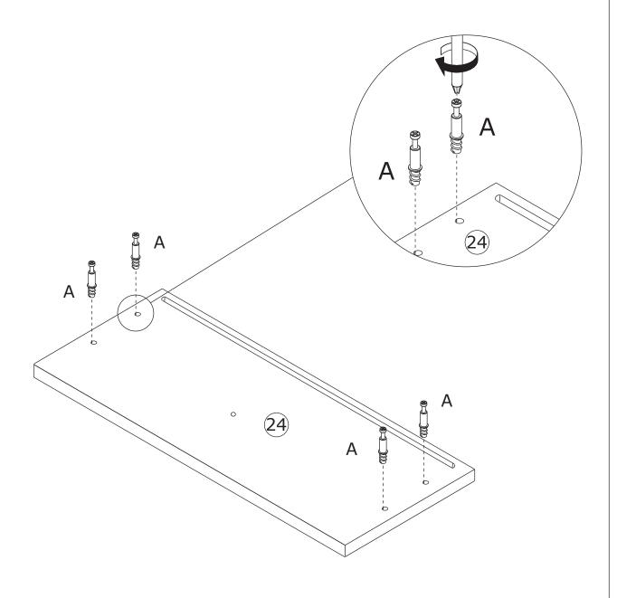
Screw eccentric rod(A) into board 24 as shown.
