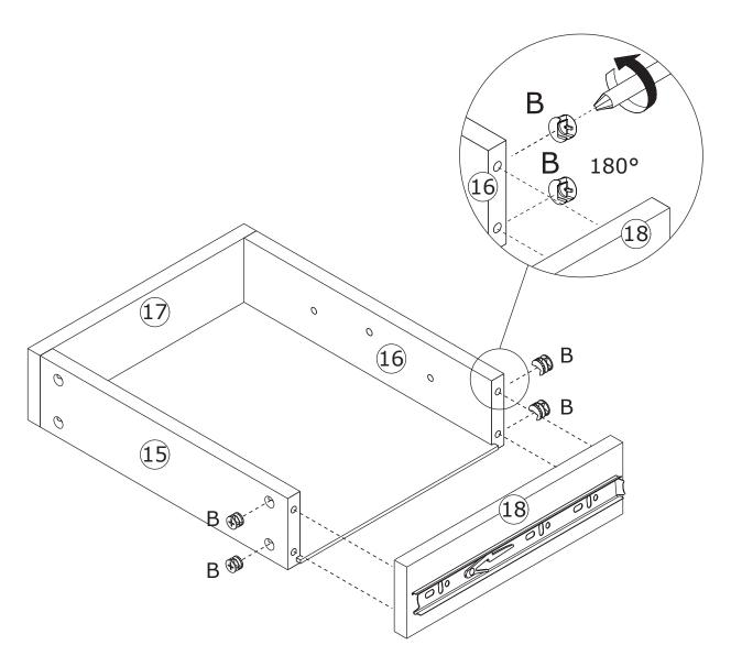
Attach board 18 to board 16 and 15, add cam lock(B) into and turn clockwise to tighten as shown.
