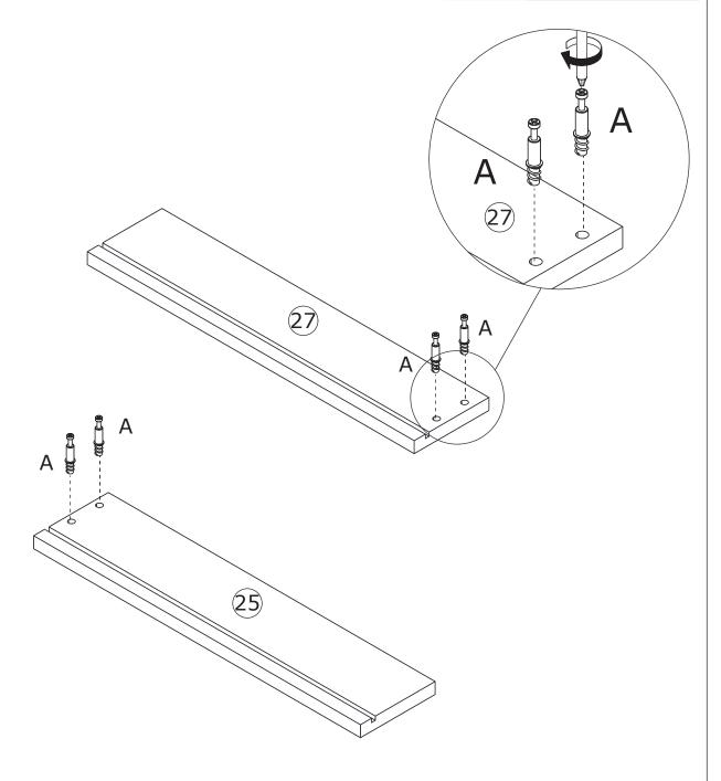
Screw eccentric rod(A) into board 25 and 27 as shown.
