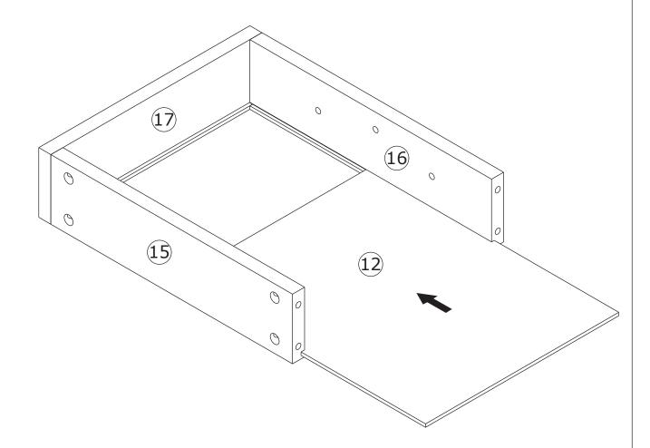
Insert bottom board 12 along grooves as shown.
