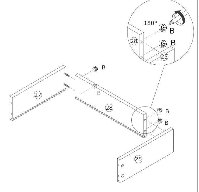
Attach board 28 to board 25 and 27, add cam lock(B) into and turn clockwise to tighten as shown.
