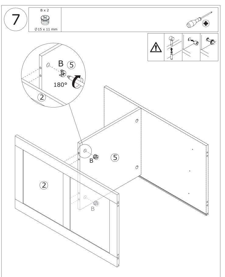
Attatch board 2 to board 5, add cam lock(B) into board 5 and turn clockwise to tighten as shown.
