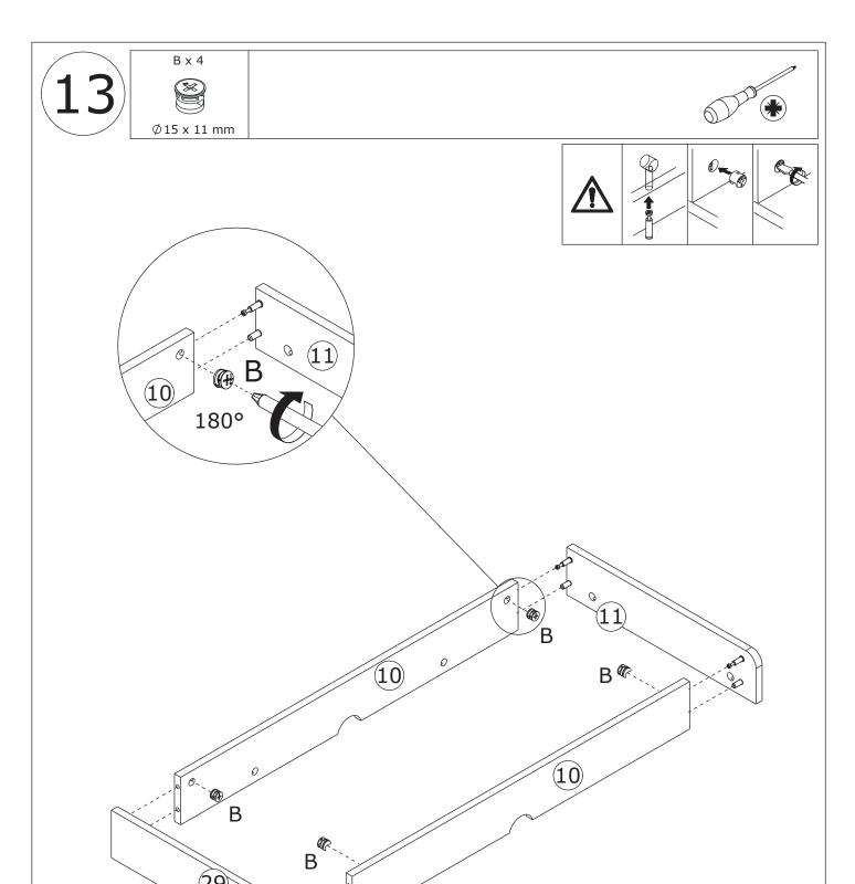
Connect board 10 to board 11 and 29, add cam lock(B) into board 10 and turn clockwise to tighten as shown.
