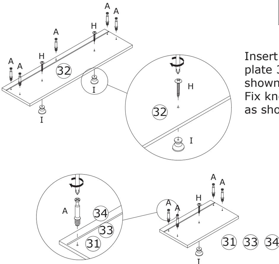
Insert quickfit screw(A) into plate 32,31,33 and 34 as shown.
