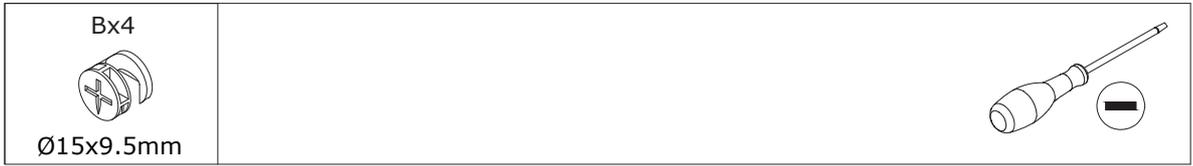
Connect plate 3 and 5 with plate 6, put cam lock(B) into holes in plate 6 and turn clockwise to tighten as shown.
