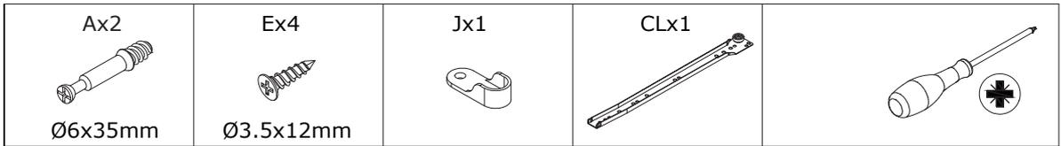
Fix slide rail(CL) to plate 4 using screw(E) as shown. Insert quickfit screw(A) into plate 4 as shown. Fix part(J) to plate 4 using screw(E) as shown.
