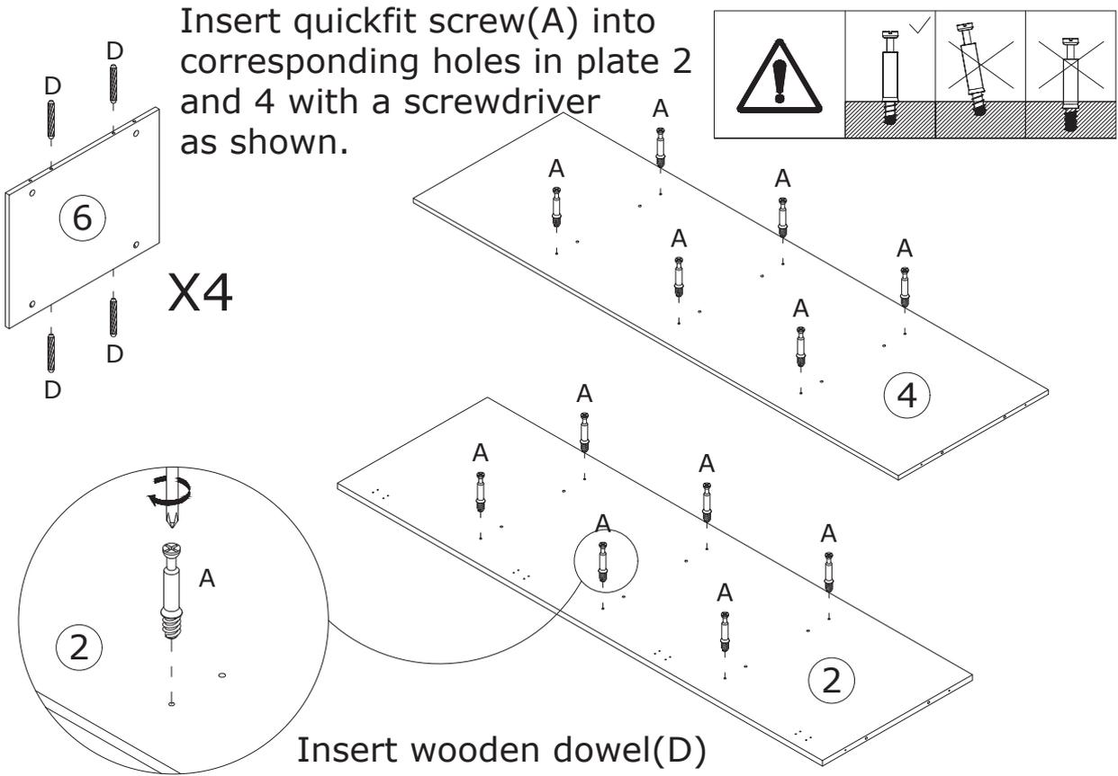
Insert wooden dowel(D) into plate 6 as shown.
