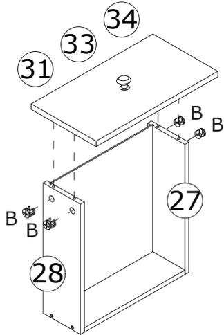
Attach plate 31/33/34 to small drawer, put cam lock(B) into holes in plate 28,27 and turn clockwise to tighten as shown.
