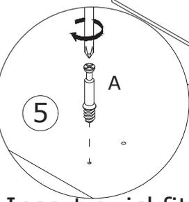
Insert quickfit screw(A) into corresponding holes in plate 3, fix part(J) using screw(E) as shown.
