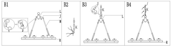
Step B1: Open the quick links (J) to attach the arm(M) to the fixture body (R) and the trim (L), Close the quick links (J)
