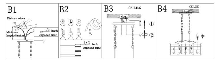
Step B1: If needed, cut off the wires length of fixture. At this point, the remaining wire length measured from the top center of canopy G is at least 6".
