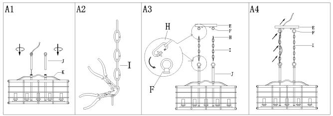
Step A1: Slip the tube (>) along wires then thread onto the nipple of top fixture body (?) till snug ,thread another tube(>) onto the nipple of top fixture body (?) till snug.
