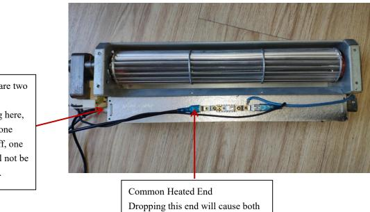
There are two sets of heating here, and if one falls off, one set will not be heated.
