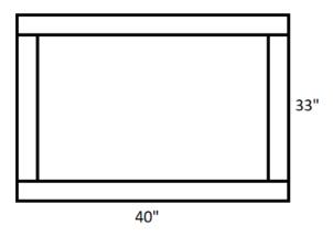
2. Cut the Category OSB for the base, 40"x36" and attach to the frame using screws or nails.
