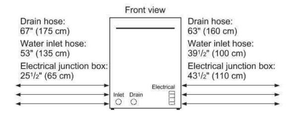
All connections in the rear of the appliance. Extensions for drain hose and electrical cord (3 pin plug) available.
