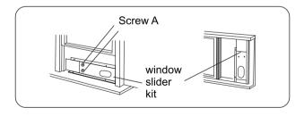
2.Attach the window slider kit to the window sash. Adjust the length of the Window Slider Kit: Loose the screw A to adjust the length of the Window Slider Kit, then tight the screw when the length is suitable.
