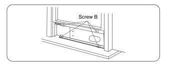
3.Carefully lower the window. Secure the vent panel in place with 4 type B screws, plus one screw for each extension.
