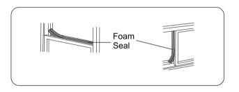
4.Cut the foam seal B(non-adhesive) to the window width. Stuff the foam seal B between the glass and the window to prevent air and insects from getting into room.
