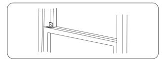
5.Install the security bracket with a type B screw, as shown.
