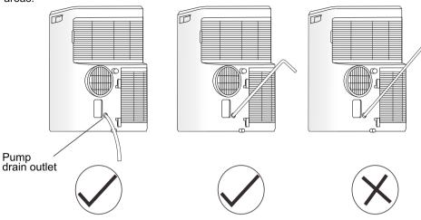
Note: Make sure the hose is secure and there are no leaks. Direct the hose toward the drain, making sure that there are no kinks that will stop the water flowing. Place the end of the hose into the drain and make sure the end of the hose is down to let the water flow smoothly. Do never let it up.
