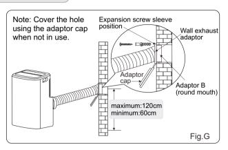
Note: 1.The duct can be compressed to 270mm minimum and extended to 1500mm maximum. It is better to keep the duct length to a minimum length.
