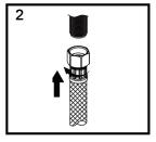
2. Attach one end of the flexible supply lines onto the shanks. Tighten the supply line connections using an adjustable or basin wrench. NOTE: Do not reuse existing supply lines.
