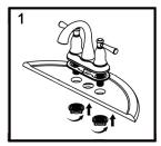
1. Place the faucet base plate to the bottom of the faucet. Run a thin bead of plumbers putty/silicone on the underside of the base plate. Insert the shanks of the faucet through the holes in the sink. From underneath the sink, thread the mounting nuts onto the shanks.Check the position of the faucet and tighten until the faucet is securely mounted. NOTE: It is helpful to have a second person hold the faucet in place while tightening the mounting nuts.
