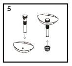
5. Apply a thin bead of putty/silicone onto the flange fig.4.1 insert the drain body into the sink slide the nut up and thread it counter clockwise on the drain body underneath the sink until it is firmly attached to the bottom of the flange Do not over tighten the nut.
