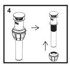
4. Install the push pop-up drain assembly: Turn the big nut clockwise to separate it from the drain body.
