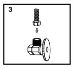
3. Attach the remaining ends of the water supply lines to the hot and cold shut-off valves and tighten with a adjustable wrench.
