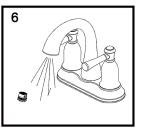
6. Remove the aerator from the spout,turn on the shut off valves. Check for leaks on supply line connections. Close the pop up assembly and fill the sink with water to check the drain for leaks. Reattach the aerator.
