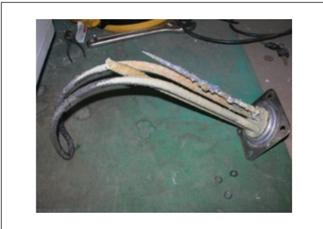
Figure 2 Depleted Anode Rod
