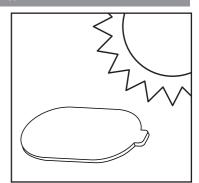
Air dry pre-motor filter for 24 hours before placing back in the vacuum.
