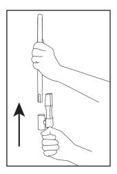
Attach crevice tool and holder by sliding it up onto the handle.
