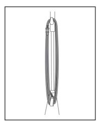
Wrap cord around the upper and lower cord wraps on the back of the vacuum. Clip plug onto the cord.
