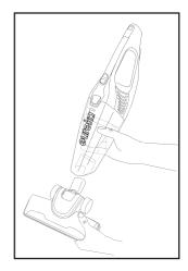
Attach the floor nozzle by inserting it into the opening at the bottom of the dust cup. Press firmly to secure in place.
