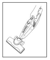
Floor nozzle may be used with the hand vacuum to clean wider surfaces
