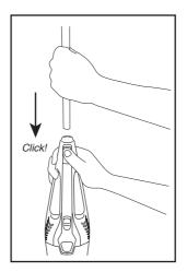
Press the quick release button on the hand vacuum grip and insert the handle. Make sure it is all the way inserted into the body of the vacuum.
