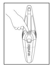
Turn on power switch on the front of the hand vacuum.
