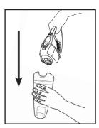
Replace filter. Attach dust cup to vacuum. Make sure dust cup is correctly secured.
