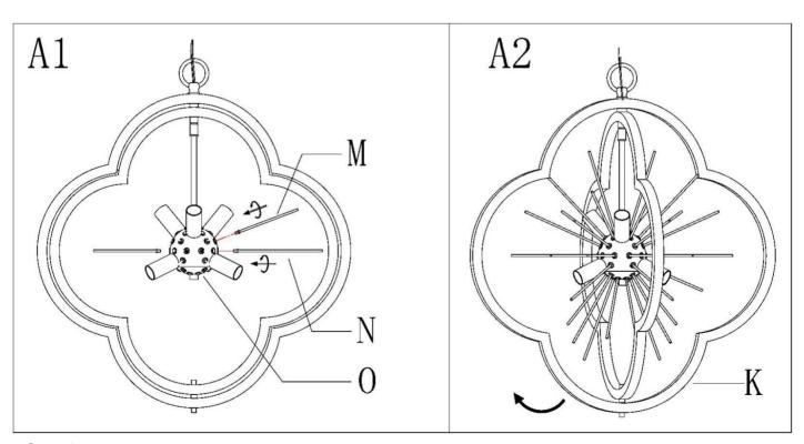
Step A1 » In staggered order, screw shorter iron bars (M) and longer iron bars (N) onto sockets assembly (O).
