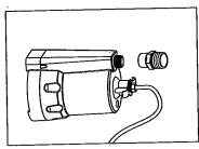
1. Attach garden hose directly to pump, OR attach the 1 1/4 in. adapter (included with pump) to pump, and then attach Hose Kit (Item #0313726) to the adapter. Slope hose away from pump to prevent backflow
