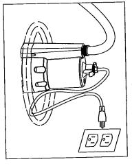
4. Allow pump to run; monitor its progress-Remove remaining water manually. has water that can drain back through the pump. Remove pump and hose from location, as hose still approximately 1/4 in. (DO NOT allow to run dry). UNPLUG when pump has removed water down to
