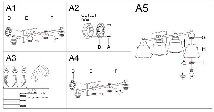
Connect wires according to the below chart
