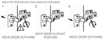
MOVE DOOR OUTWARD by turning this screw counter-clockwise
