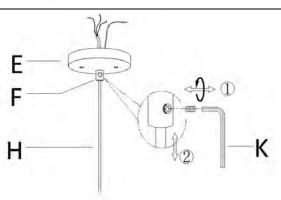
5. If needed, shorten the extra length of the fixture wires through the cord (H) so that they all are at least 6 inches (152.4 mm) long above the canopy (E) within the outlet box.
