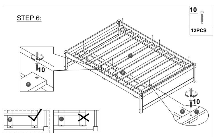
Note: Do not lock the screws of the bed slats to the outermost edge of the bed slats, you need to leave a certain space at the edges, otherwise it will cause the board to break
