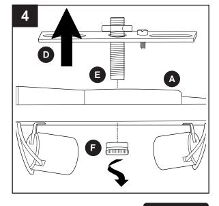
5. Attach mounting strap (D) to outlet box (not included) using the existing screws and washers.
