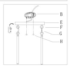
5. Attach the mounting plate(B) to outlet box with the mounting screws(D)
