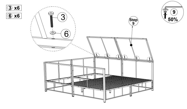
Connect the part from step 18 & the part from step 9, tighten Bolt (3) & Flat Washer (6) with Allen Key (9).
