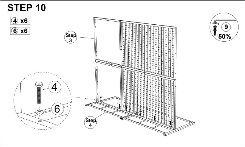
Connect The part from Step 3 & The part from Step 4, tighten Bolt (4) & Flat Washer (6) with Allen Key (9).
