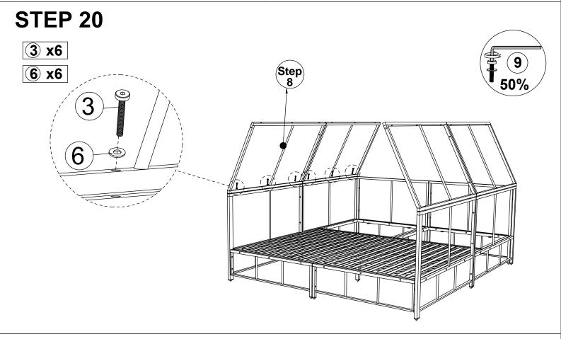
Connect the part from step 19 & the part from step 8, tighten Bolt (3) & Flat Washer (6) with Allen Key (9).
