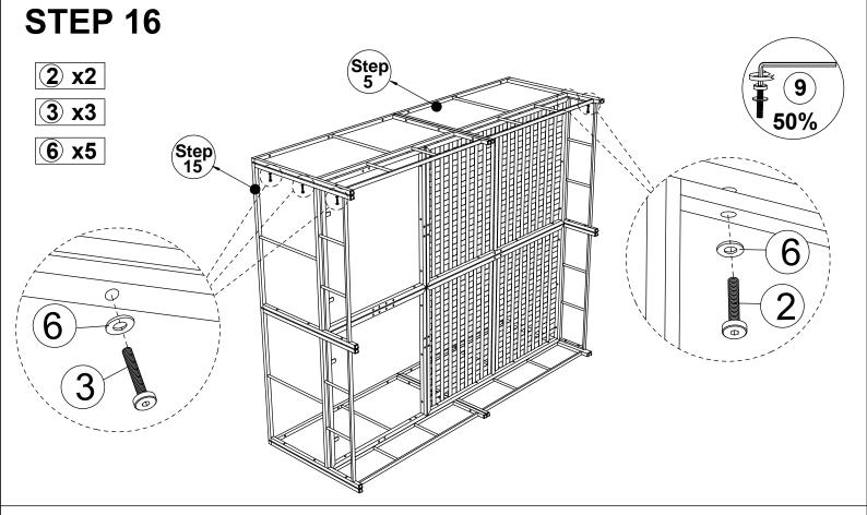
Connect the part from step 15 & the part from step 5, tighten Bolt (3) & Bolt (2) & Flat Washer (6) with Allen Key (9).
