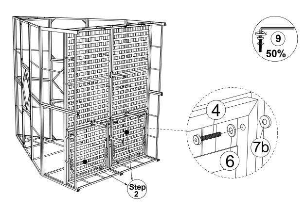
Connect The part from Step 33 & The part from Step 2, tighten Bolt (4) & Flat Washer (6), Plastic Washer (7b) with Allen Key (9).
