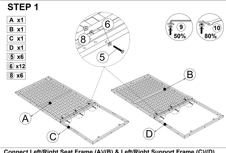
Connect Left/Right Seat Frame (A)/(B) & Left/Right Support Frame (C)/(D), with tighten Bolt (5) & flat washer (6) & Eru (8), Allen Key (9) & Key (10).
