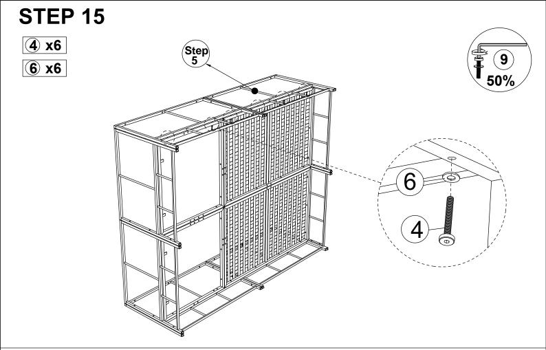
Connect the part from step 14 & the part from step 5, tighten Bolt (4) & Flat Washer (6) with Allen Key (9).
