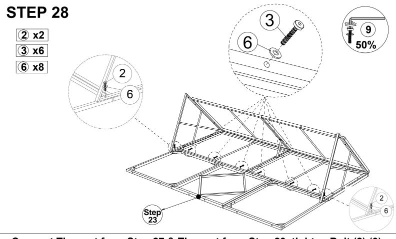
Connect The part from Step 27 & The part from Step 23, tighten Bolt (2),(3) & Flat Washer (6) with Allen Key (9).
