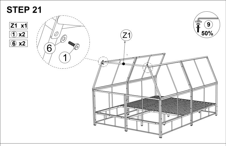
Connect the part from step 20 & Support Bar 1(Z1), tighten Bolt (1) & Flat Washer (6) with Allen Key (9).
