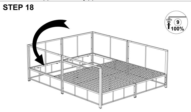
Turn the part from step 17 upright, firmly tighten Bolts with Allen Key (9)
