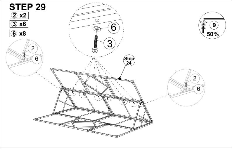
Connect The part from Step 28 & The part from Step 24 With tighten Bolt (2), (3) & Flat Washer (6) with Allen Key (9).
