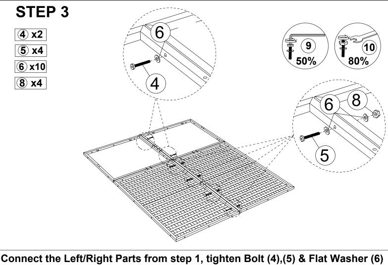
Connect the Left/Right Parts from step 1, tighten Bolt (4),(5) & Flat Washer (6) & Allen Key (9) & Key (10).
