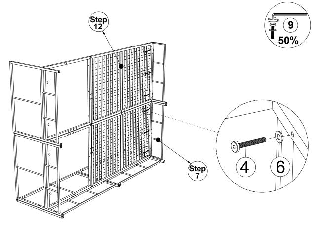
Connect the part from step 12 & the part from step 7, tighten Bolt (4) & Flat Washer (6) with Allen Key (9).
