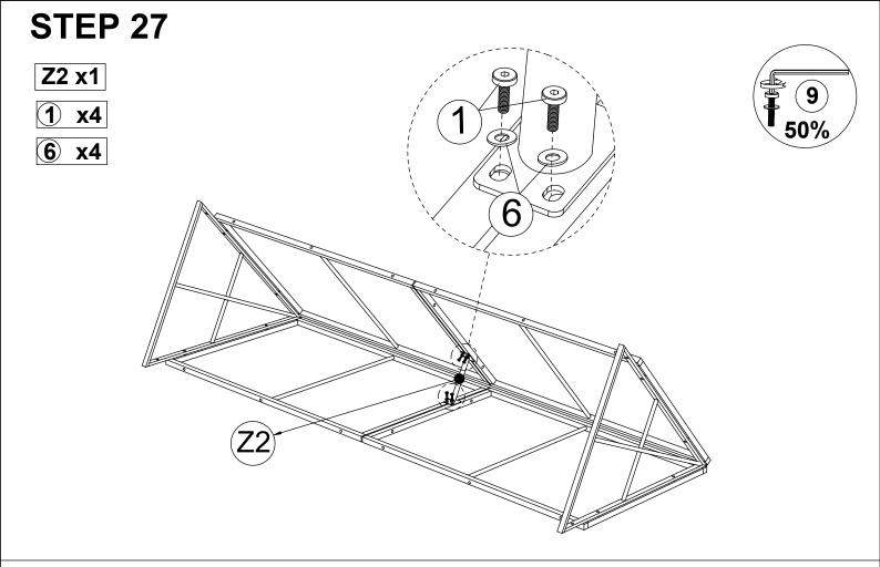
Connect a part from Step 26 & Support Bar (Z2), tighten Bolt (1) & Flat Washer (6) with Allen Key (9).
