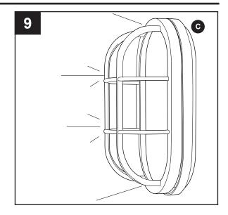
10. After completing installation, caulk fixture (C) mounting surface with silicone weather sealant (not included).
