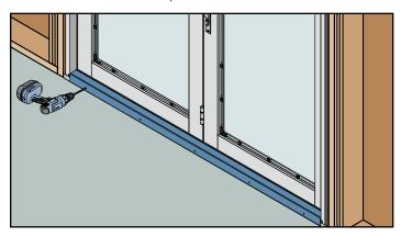
3. Remove and apply a 1/8" bead of sealant to the backside of the sill screen adapter where it will contact the top of the threshold.
