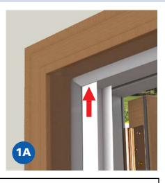
Next, install the Top Guide (A on page 2) by tucking each end into the Side Guides and centering it in the frame. Secure with # 8 x 3/4" Phillips Screws in the predrilled holes (1B below).
