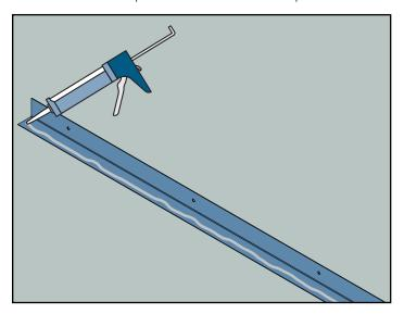
4. Apply the sill screen adapter to the interior threshold of the wall system and fasten using the provided #8 x 1/2 " pan-head screws. **NOTE:** To avoid stripping, **ONLY** tighten until snug.
