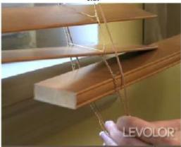
Step 7: Pull the lift cord out of the last loop on the ladder cord below the bottom rail (repeat for all lift cords)
