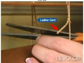
Step 4: Cut both lift cords approximately 6 in. below the new bottom slat (repeat for all sets of lift cords)
