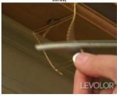
Stuff any remaining ladder cords into the bottomrail and reinsert the plugs seating the cords in the plug notches (repeat for all ladder cords)
