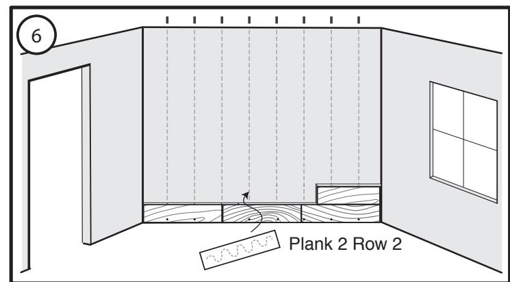
Tighten long side joints as needed with a tapping block or pull bar. Drive a brad nail into each plank through the shallow area of the extended groove at each wall stud. Repeat this process for the remainder of row 2, being sure to cut the last plank to leave a 3/16" gap against the adjoining wall. (Figure 7)
