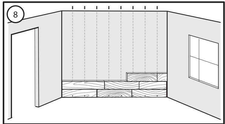
For the last row of the installation, use painters tape to mark the stud location for brad nailing. Cut the planks for the last row to the correct width and complete the installation as you have the earlier rows. (Figure 8A)
