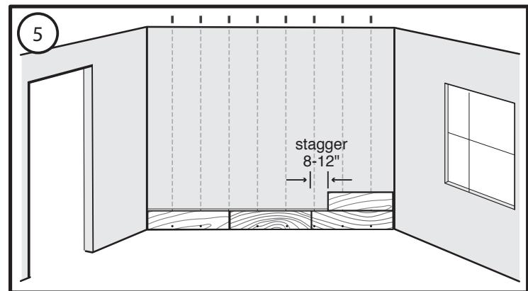
For plank 2 of row 2 (and each plank thereafter in row 2), first apply silicone adhesive caulk in an "S" pattern to the back of the plank. Insert the long side tongue into the long side groove of row 1. While holding plank 2 at approximately a 45 degree angle to the wall, slide plank 2 of row 2 to the right until the short end just touches the short end of plank 1 in row 2. Rotate plank 2 towards the wall to engage both the long side and short side joints. (Figure 6)
