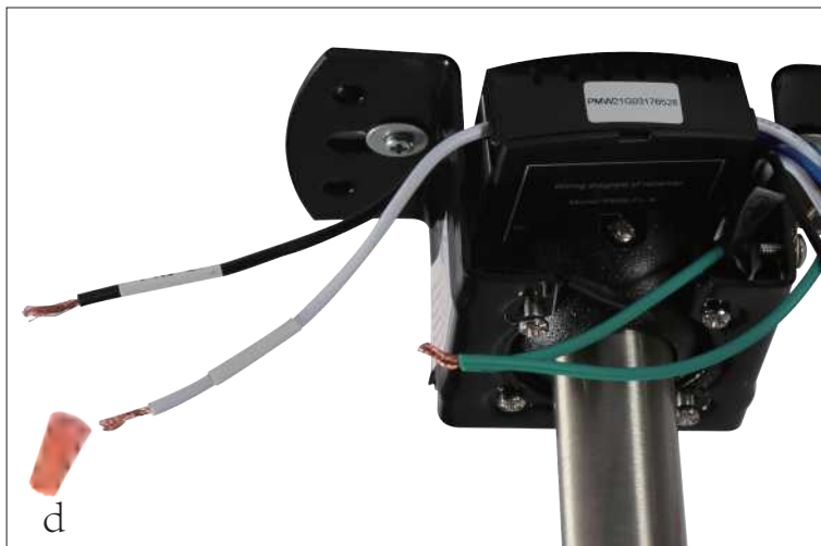
Step 13 Connect the receiver to home wires. Black for Live wire, White for neutral wire, Green for ground wire.
