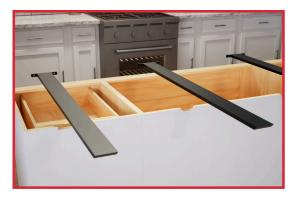
2. Once your kitchen island cabinet is notched, place your brackets in the notch. Slide your brackets into place against the top stretcher. Ensure the top of the bracket is flush and level with the top of the cabinet.
