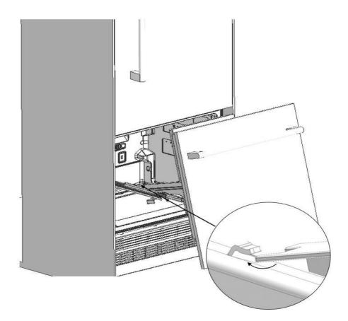
• Fix the Freezer Furniture door assembly onto the rails with 2 screws.
