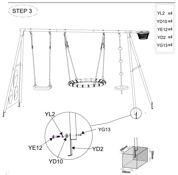
WARNING: The anchors must be placed under the ground in order to reduce tipping hazards
