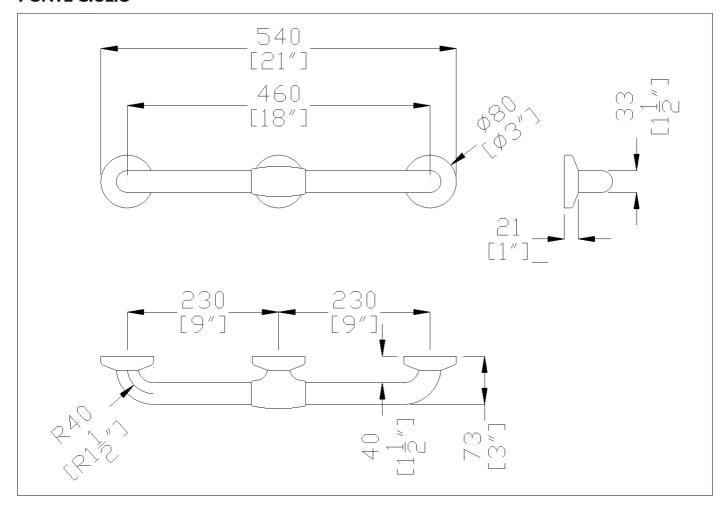
Bariatric 18" antimicrobial vinyl coated grab bar. No maintenance 3mm thick antimicrobial vinyl coating. Concealed stainless steel 11-hole flange plate.
