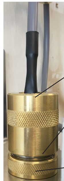
2) Quartz Sleeve inserted into UV Chamber Quartz Sleeve Black O-Ring Locking Nut
