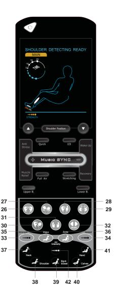
The Remote Control is divided into 4 main sections with different functional purposes. The pages that follow describe the functions of the various buttons within these sections.
