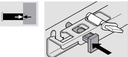
Lock the peg by pushing inside the hole in the drawer base side.
