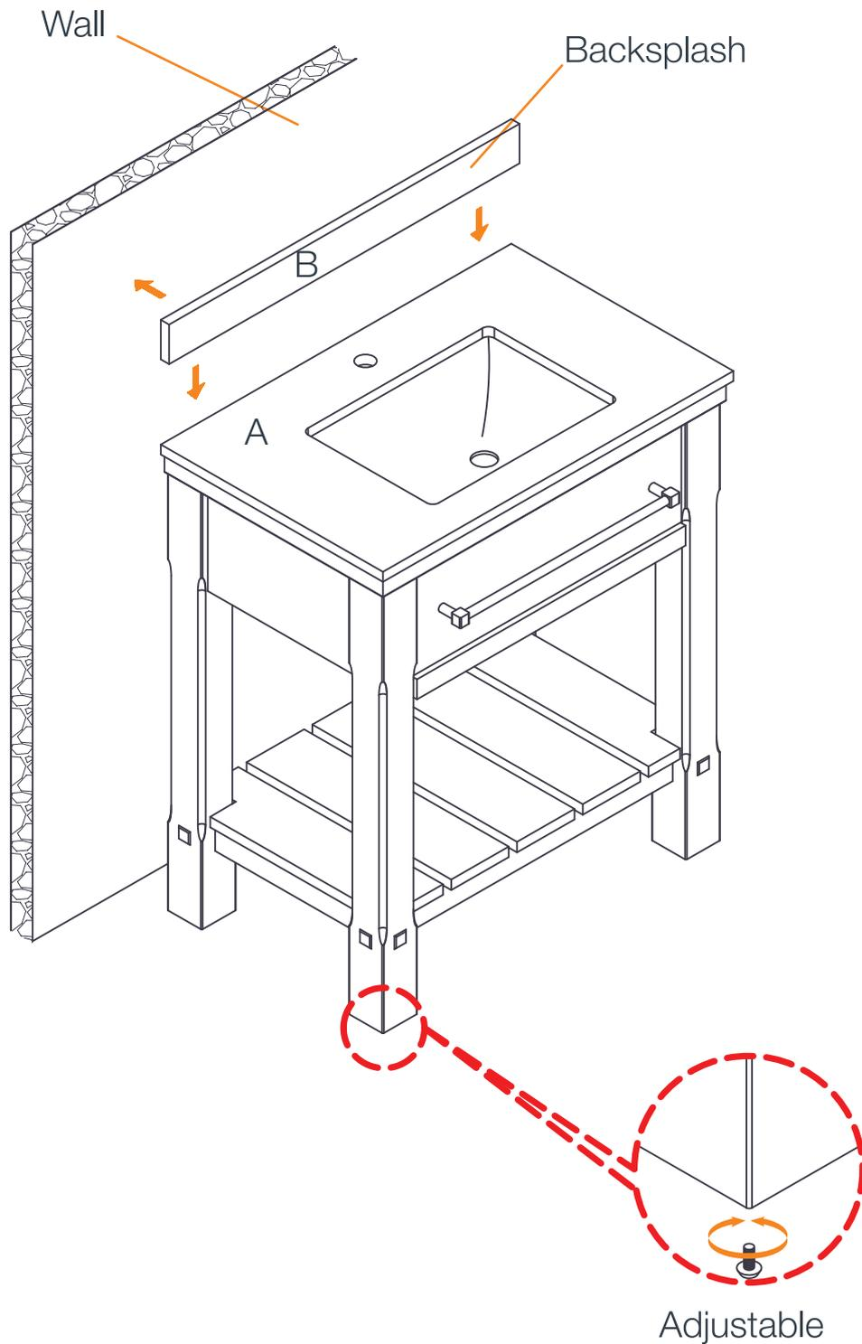
For application of backsplash (B) to drywall: Make sure the wall is smooth and flat. Clean the wall and the back of the backsplash (B) with damp cloth to remove any grease or debris. Apply thin-set adhesive, and then set the backsplash (B).
