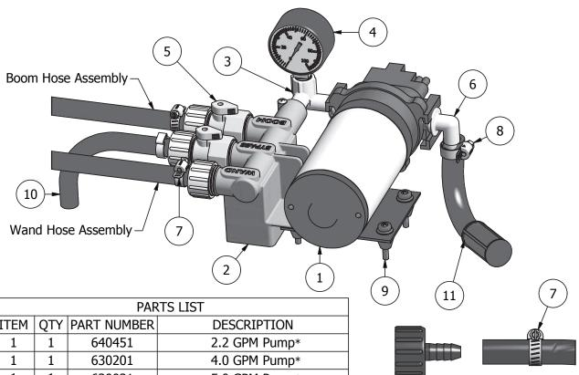
ITEM 5.0 GPM Pump\* Manifold Body Elbow (2.2 pumps) Elbow (4.0 & 5.0 pumps) Gauge 0-100 PSI Inline Valve **QD EL 12** 5/8" Hose Clamp 1/2" Hose Clamp 10-24 x 1.25 Screw Relief Hose Assembly **Suction Hose Assembly** Cap Assembly (not shown)
