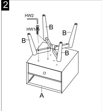
Step 2: Attach the 4\*legs (B) to the bottom side of Drawer (A), And use the Allen Key (HW2) to lock with 8\*Hex Socket Bolts (HW1), as picture.
