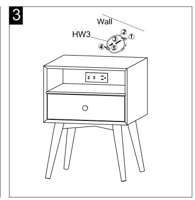
Step 3: Straighten up the assembled product. Following the installation instructions of anti-tipping (HW3) to fix the product in the wall by strap. Assembly is completed.
