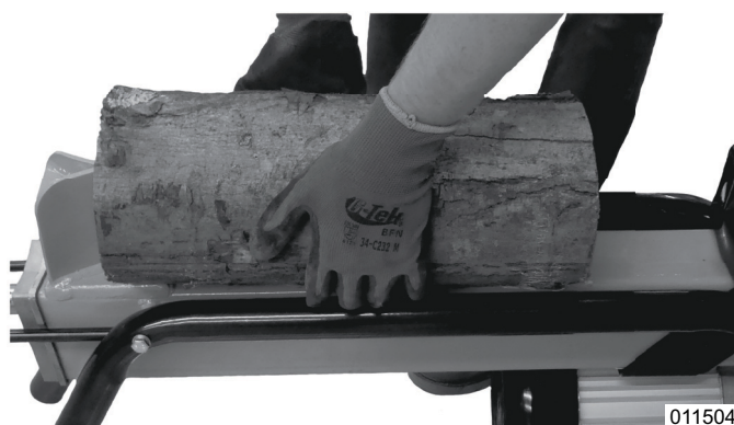
Figure 3-5. Correct Log Loading Technique
