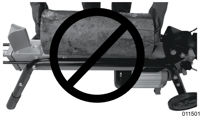
Figure 3-2. Do Not Hold at Ends
